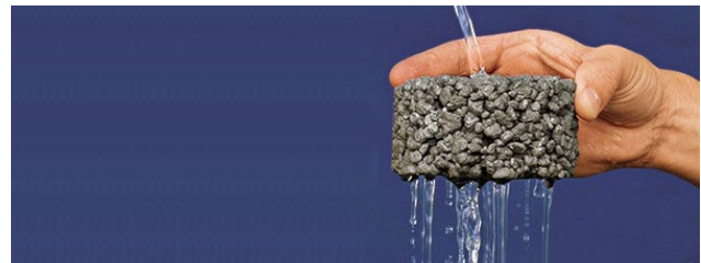
Figure 6. A Visual Representation of Hydraulic Conductivity: A measure of how easily water moves through soil and aquifer materials (Image from Build LLC 2013).
