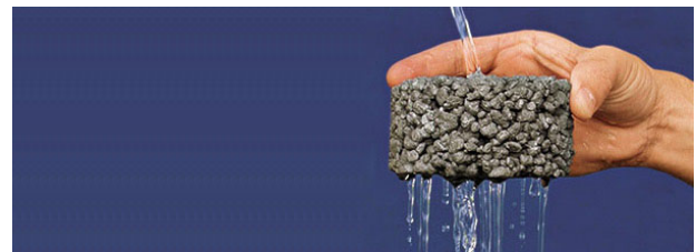
Figure 3. A visual representation of hydraulic conductivity: a measure of how easily water moves through soil and aquifer materials (Image from Build LLC 2013).
