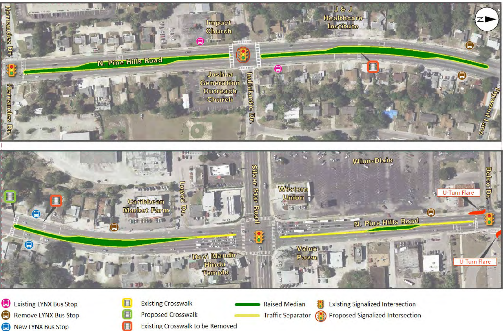
Figure 2.3 (continued): Build Alternative - Raised Median Concept
